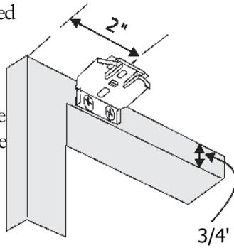
front clip of the bracket into the front groove of the rail.
